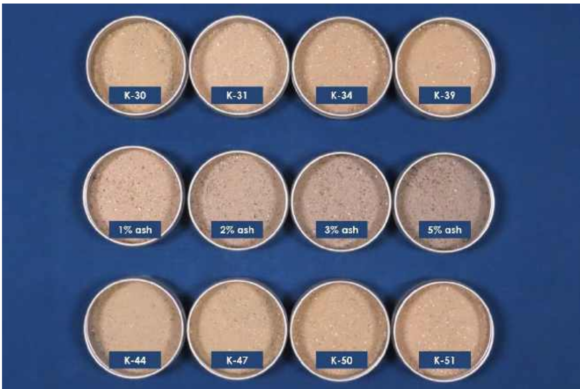
Figure 10 – Comparison of processed Class II sand type samples to select reference standards (middle row).
