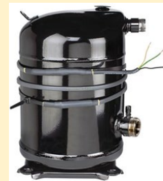
Figure 23: “Belly Band” crankcase heater (heating wire wrapped around compressor).
